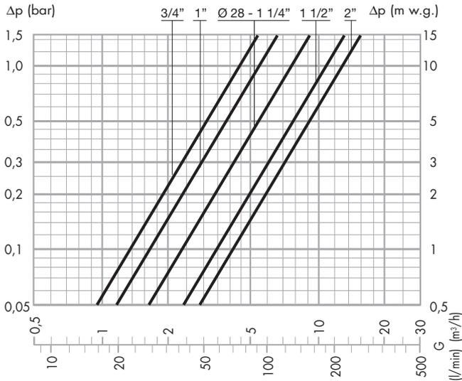
**Recommended FLOW RATES to ensure stable operation and accuracy of  $\pm 2^\circ\text{C}$  (balanced Hot/Cold pressures)**
